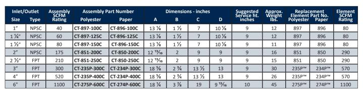
Note: CT 2" & 2 ½" models: element seals on the base of the housing. \*See Vacuum Filter Technical Data for vacuum service data and sizing guidelines.
